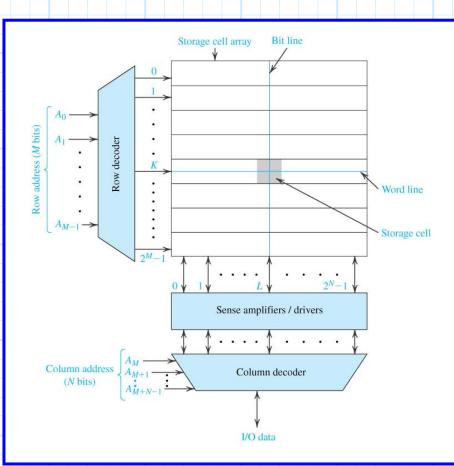
Thus, we can say that typically a semiconductor memory is an arrangement of  $2^{M}$  rows, with each row consisting of  $2^{N}$  storage cells.
